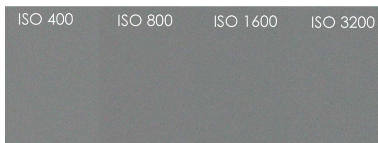
Figure 1. Images captured on my 700D at different ISO settings. The shutter speed and aperture were exactly the same for each image: 1/50 sec at f8. The camera’s high ISO NR was turned off. The images were post-processed to correct for the under- or overexposure. Each panel is a 1:1 crop from the original (ie. each pixel in the panel represents a pixel in the original image).
