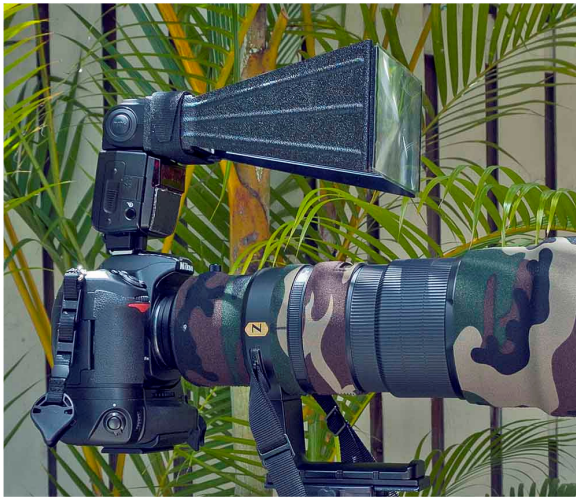
Better Beamer Flash Extender mounted on a Nikon SB-600 Speedlight and Nikon D300 camera. The lens is a Nikon 500 mm AF f4 with VR
